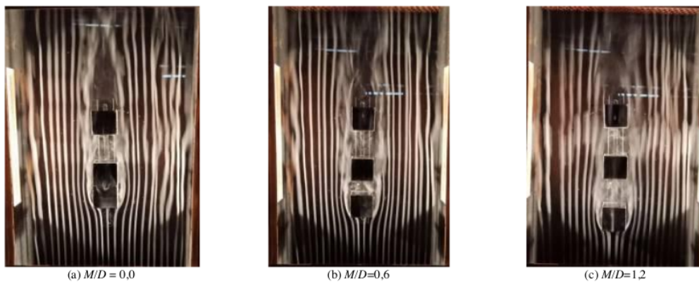
Figs. 6. Visualization of flow in three tandem square cylinder in model I serial configurations or (a) M/D=0.0 ; (b) M/D=0.6 and (c) M/D=1.2 while N/D is constant at 1.2 at Re=43,844
