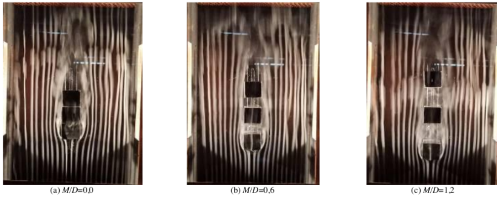
Figs. 7. Visualization of flow in three tandem square cylinder in model II serial configurations or (a) M/D and N/D=0.0 ; (b) M/D and N/D=0.6 and (c) M/D and N/D=1.2 at Re=43,844
